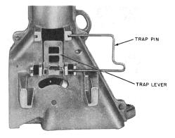
Fig. 48—Placing Trap Lever Pin on Hopper
