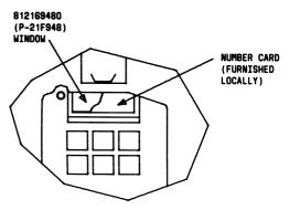
FIG. 2 — Window and Number Card Installed in Faceplate (TOUCH-TONE Set)
