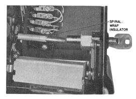
Fig. 10—Cutaway Section of Upper Housing Showing Mating of Bolt Fastener and KS-19277 Lock
