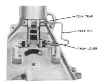
FIG. 3 — Placing Coin Trap in Hopper
