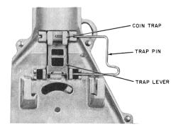
Fig. 49—Placing Coin Trap in Hopper
