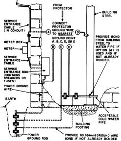
Fig. 4—Acceptable Water System—MGN Power Service Grounded to Ground Rod
