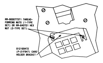
FIG. 3 — Card Holder Bracket Installed (TOUCH-TONE Set)
