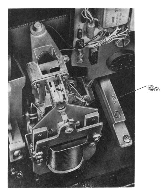
Fig. 6—Installation of Drilling Template
