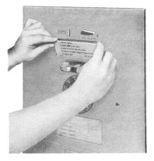
FIG. 3 — Installing Instruction Cards In Early Production 2-Type Set
