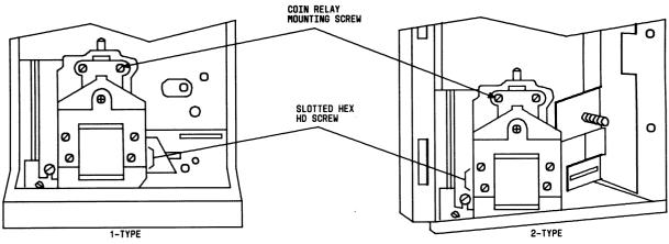
FIG. 1 — Housing and Mounting Plate Assembly
