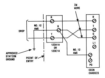
FIG. 2 — Protector Wiring When Protector is Inside Set
