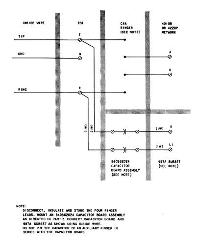
Fig. 53—Optional Ringer Connections
