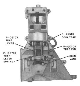
Fig. 2—♦Coin Trap and Trap-Lever Assembly♦
