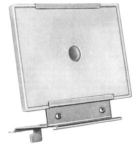
Fig. 21—Securing Instruction Card (Typical)
