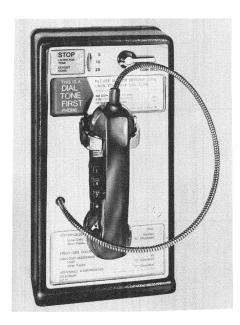
Fig. 37—Coin Cover Unit With Handset Inverted
