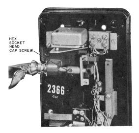
Fig. 27—Method of Securing Adapter to Switchhook Assembly
