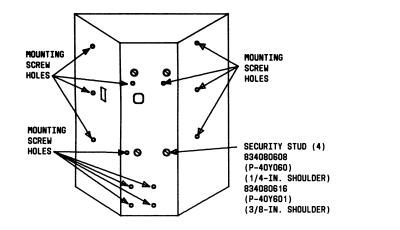
FIG. 1 — Location of Mounting Screw Holes and Security Studs In 2D-Type Set
