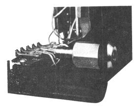
Fig. 4-KS-19277 Lock Installed in Upper Housing
