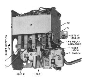
Fig. 14—Checking Totalizer Rate (Typical)
