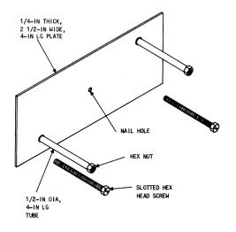
Fig. 8—**\**Twin-Bolt Fastener**(**
