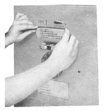
FIG. 3 — Installing Instruction Card In Early Production 2-Type Set
