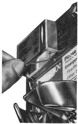
Fig. 57—Setscrew Adjustment
