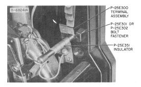
Fig. 7—Terminal Assembly, Insulator, and Bolt Fastener
