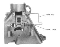
FIG. 2 — Placing Trap Lever Pin in Hopper
