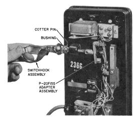
Fig. 26— Installation of Adapter Assembly and Switchhook Assembly
