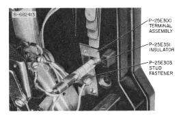
Fig. 6-Terminal Assembly, Insulator, and Stud Fastener
