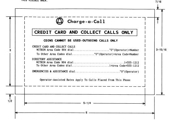
Fig. 11—Instruction Card for KS-22284 Backboard (Typical)
