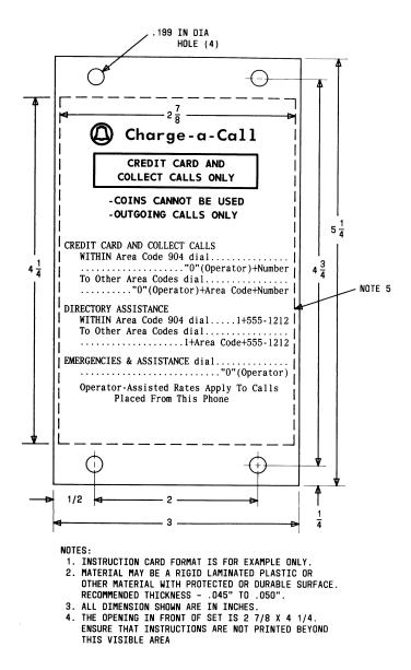
Fig. 7—Instruction Card for 10A or 20A Coinless Telephone Set (Typical)
