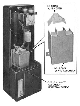
Fig. 29—Relay Antidrill Guard Arrangement
