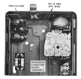
Fig. 51—Housing and Mounting Plate Assembly
