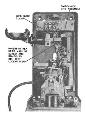
Fig. 22— Switchhook Installed
