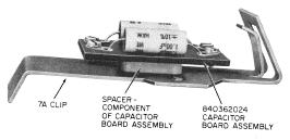
Fig. 52—Capacitor Board Assembly Mounted on 7A Clip
