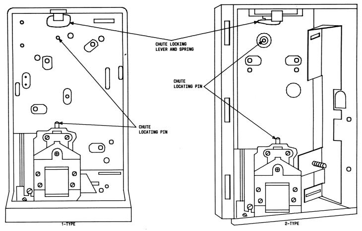
FIG. 2 — Housing and Mounting Plate Assembly
