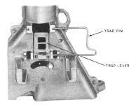
FIG. 5 — Placing Trap-Lever Pin in Hopper
