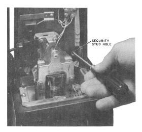
Fig. 8—Determining Presence of Keyhole Slots
