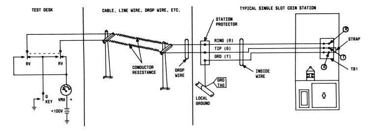
FIG. 1 — Ground Resistance Measurement
