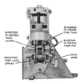
Fig. 47—Coin Trap and Trap Level Assembly
