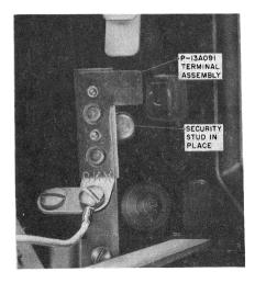
Fig. 5—P-13A091 Terminal Assembly with Security Stud Installed
