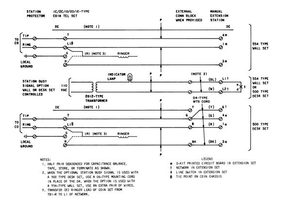
Fig. 1—Connections for Manual Extension Station Service With Station Busy Signal Option in Association With Semi-Public Coin Telephone Set
