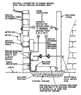
Fig. 3—Acceptable Water System or Building Ground—Power Service Grounded to Building Footing Ground
