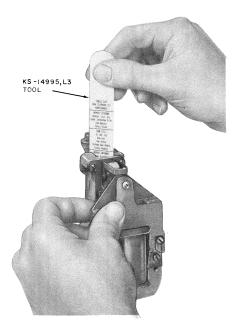
Fig. 38—Trap and Vane Release Test
