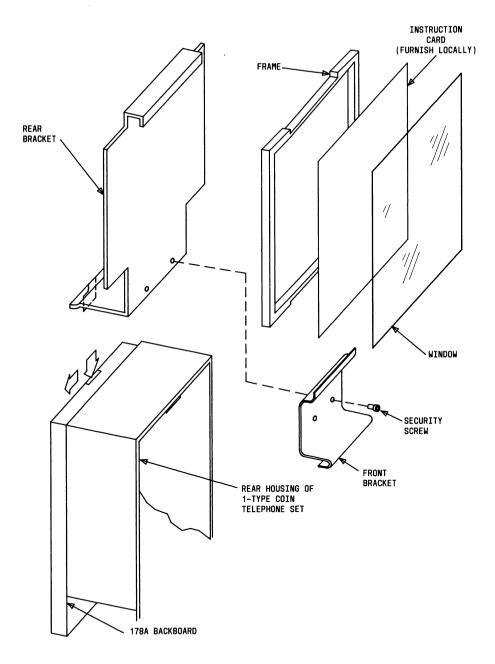
Fig. 23—Installation of 11A Card Holder
