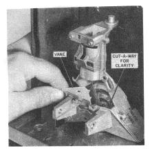
FIG. 3 — Inserting Vane
