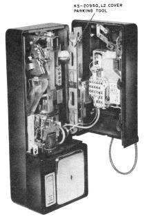
FIG. 1 — 1D-Type Coin Telephone Set With Parking Tool Installed
