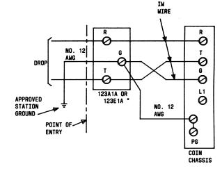
FIG. 3 - Protector Wiring When **Protector is Inside Set**
