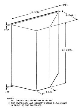
Fig. 3—Rear View of Panel Set Showing Dimensions
