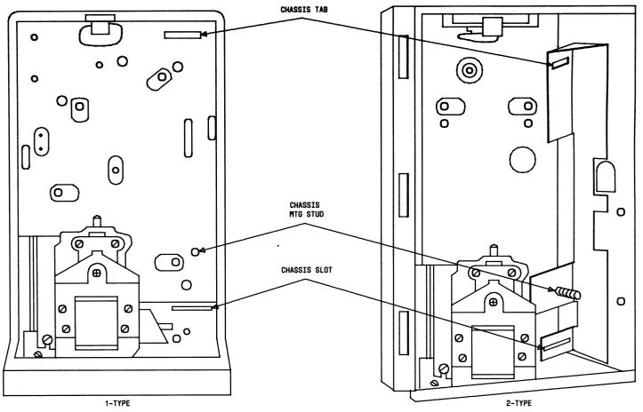
FIG. 1 — Housing and Mounting Plate Assembly
