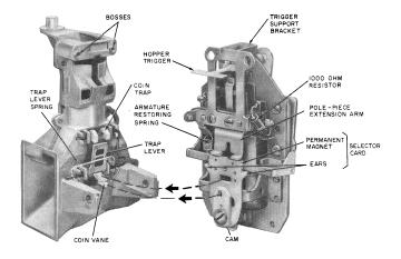
FIG. 2 - Coin Hopper and Rear View of Coin Relay
