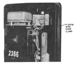
Fig. 25—Installation of Wire Guide Clamp
