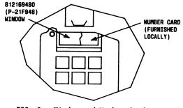
FIG. 3 — Window and Number Card Installed in Faceplate (TOUCH-TONE Set)
