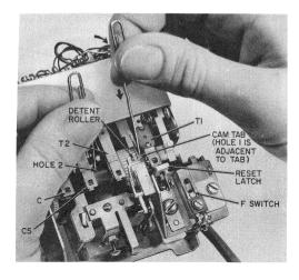
Fig. 15—Increasing Totalizer Rate (Typical)
