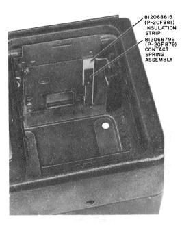
Fig. 7—)Installation of Insulation Strip and Contact Spring Assembly(
