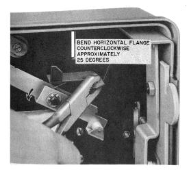
Fig. 61—Bending Chute Guide (Limit Stop)
