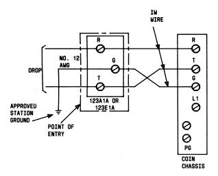
FIG. 2 - Protector Wiring When Protector is Outside Set
