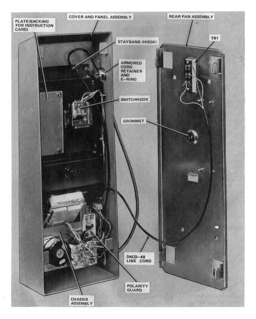
Fig. 4—10A Coinless Telephone Set With Rear Pan Assembly Removed
