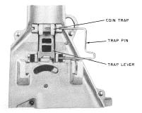
FIG. 6 — Placing Coin Trap in Hopper
