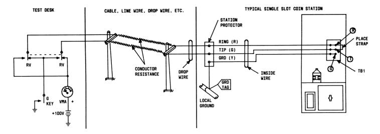
FIG. 1 - Loop Resistance Measurement
